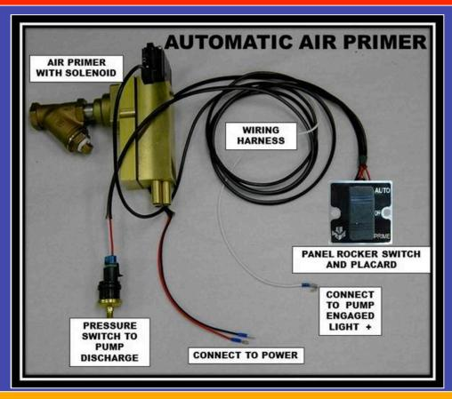
The test primer was the new, Automatic Air Primer made by Trident Emergency Products. The primer was installed on E142 by 4-Guys.
