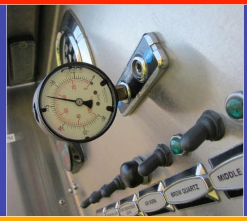
The vacuum gauge displayed a reading of 13-inches which equaled 14.7 feet of lift.
