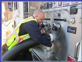
35-feet of 6-inch hard suction hose was connected to the driver side 6-inch suction intake on Engine 142. The other end of the suction hose was connected to a 6-inch Kochek low level strainer and placed into the stream.
