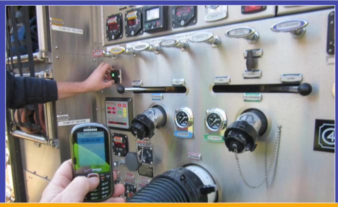
Time was started when the driver pushed the air primer's control switch and stopped when discharge pressure was observed on the master discharge gauge.
