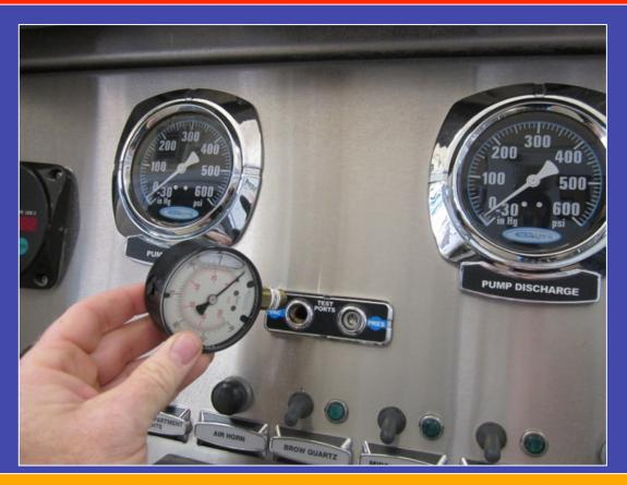
A vacuum gauge was connected to the pumper's vacuum test port for accurate measurement of lift. The gauge was graduated in 1-inch increments.
