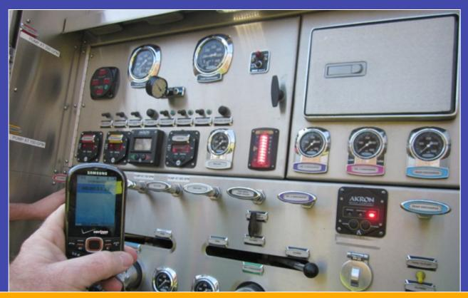
At the 53-second mark, discharge pressure was observed on the master discharge gauge and the pump was primed! Flow was started out the deck gun.
